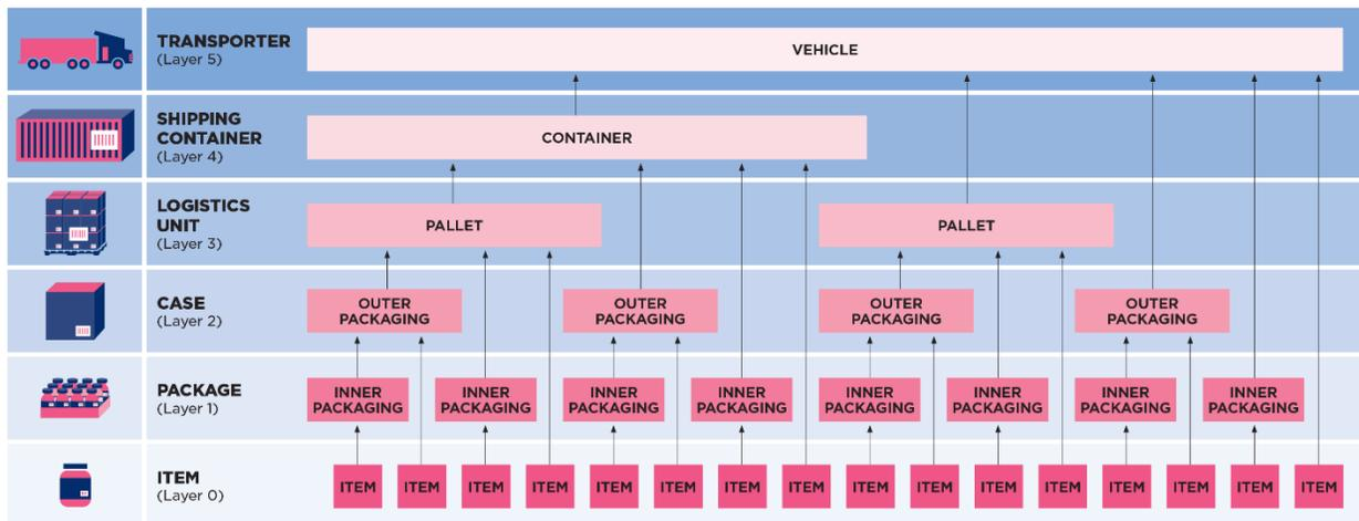
Figure 1: Typical Transport Hierarchy – example of cargo layers
